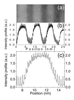
FIG. 3 (a) High resolution Z-contrast image of the QCD structure prepared by <100> crosssection; (b) Corrected intensity profile along the growth direction. (c) Zoom of the intensity profile over two interfaces.
