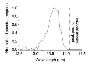
FIG. 10 Spectral response of the QWIP in presence of a inhomogeneous distribution of charges. 700 distributions of charges have been evaluated to obtain this graph.
