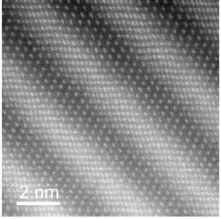
FIG. 2 High resolution Z-contrast image of the  $9\mu m$  QCD structure prepared by <100> cross-section.
