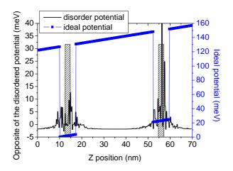
FIG. 9 Opposite of the disordered potential for a given distribution of charge (N=15 charge per well-R~40nm). The striped pattern shows the doping position.
