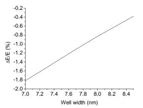
FIG. 6 Difference of the energy transition with and without non-sharpness, normalized by the initial transition energy  $\left(\frac{E_{non-sharpness} - E_{ideal}}{E_{ideal}}\right)$ , as
