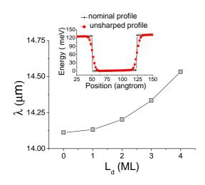
FIG. 4 Evolution of the wavelength associated to the transition between the ground state and excited state as a function of gradient extension in monolayers (ML). Inset: EBP from a single well for  $L_d=2ML$  and  $F=5kV.cm^{-1}$ .
