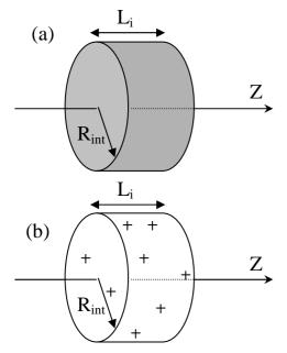
FIG. 8 (a) volume of integration of the screened potential in the case of an homogenous volume distribution, (b) volume of integration of the screened potential in the case of a discrete distribution.
