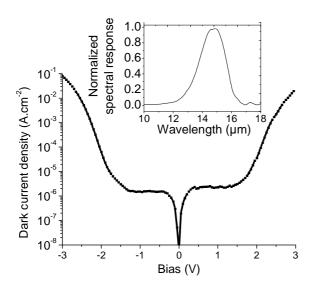
FIG. 1 Dark current as a function of the voltage bias at T=4K. Inset: normalized spectral response at T=4K and V=-1V.
