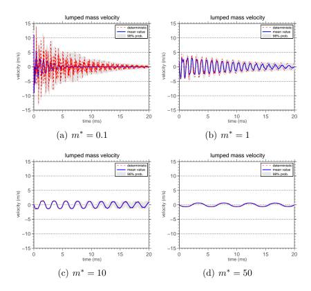
Figure 5: This figure illustrates the mean value (blue line) and a 98% of probability interval of confidence (grey shadow) for the random process  $U(L, \cdot, \cdot)$ , for several values of the discrete–continuous mass ratio.
