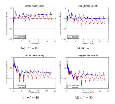
Figure 7: This figure illustrates estimations to the PSD of the random process  $U(L, \cdot, \cdot)$ , for several values of the discrete–continuous mass ratio.
