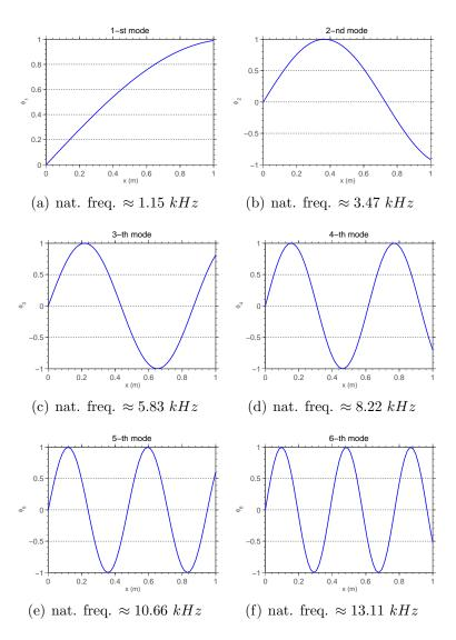
Figure 3: The first six orthogonal modes and the corresponding (approximated) natural frequencies of a fixed-mass-spring bar with  $m = 1.5 \ kg$ .
