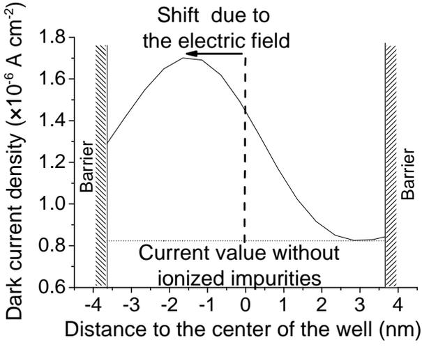
FIG. 8. Dark current density (full line) as a function of the doping position in the well, under an electric field of  $10 \text{ kVcm}^{-1}$ . The dotted line is the current value for the same electric field but without ionized impurities.
