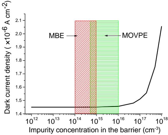
FIG. 11. Dark current density as a function of the concentration of undesired ionized impurities in the barrier under an electric field of  $10\text{kVcm}^{-1}$ . The two rectangles highlight the typical range of concentration for MBE (leaned pattern) and for MOVPE (horizontal pattern)
