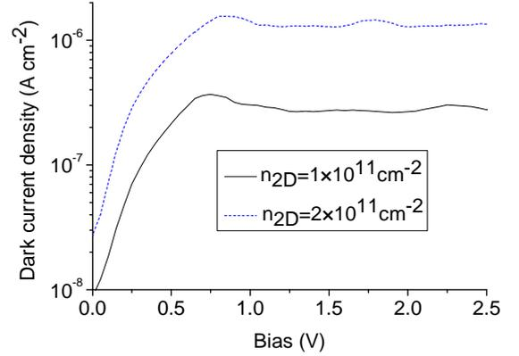
FIG. 7 Dark current as a function of the applied bias for component B<sub>1</sub> (doping level of  $1 \times 10^{11} \text{cm}^{-2}$ ) and B<sub>2</sub> (doping level of  $2 \times 10^{11} \text{cm}^{-2}$ ).
