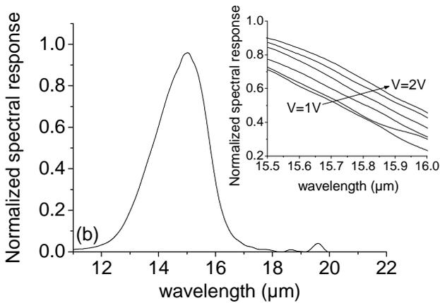
FIG. 1(a) Dark current density as a function of the applied bias for  $T=4\text{K}, 10\text{K}, 20\text{K}, 30\text{K}, 40\text{K}, 50\text{K}$  and  $60\text{K}$ . (b) Spectral response at  $T=10\text{K}$  for  $V=1.5\text{V}$ , inset spectral response for different bias voltages from  $V=1\text{V}$  to  $V=2\text{V}$  by step of  $0.2\text{V}$ , in the  $15.5\mu\text{m}-16\mu\text{m}$  range.
