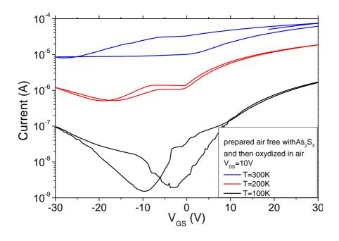
Figure S 5: drain source current as a function of the gate source bias, for a 10V drain source bias at different temperature. The film has been processed in the glove box with  $As_2S_3$  and then oxidized by removing the film from its cell and then being heated under heat gun.
