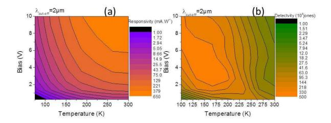
Figure S 6 (a) and (b) are the responsivity and detectivity map as a function of bias and temperature of a film of HgTe CQD treated with  $As_2S_3$  and a cut-off wavelength at  $2\mu m$ .
