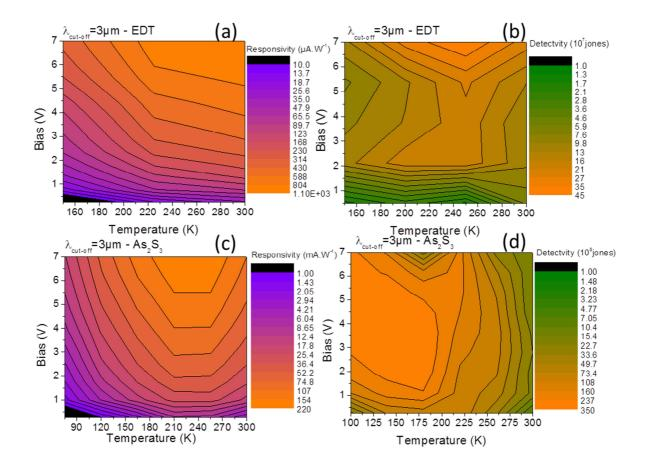
Figure 3 (a) Responsivity map as a function of bias and temperature for a film of HgTe CQD treated with ethanedithiol. (b) Detectivity map as a function of bias and temperature for a film of HgTe CQD treated air free with ethanedithiol. (c) and (d) are respectively the responsivity map and detectivity map of the same HgTe CQDs but processed with  $As_2S_3$  at 1kHz.
