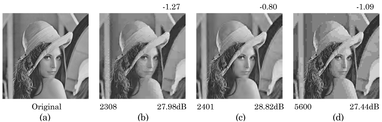
Figure 7. Image compression comparison of Lena image (a) Original Image, Image compressed by (b) ICA, (c) JPEG2000, (d) JPEG (Image size is at bottom left(in bytes), PSNR is at bottom right and PQS is at top right).
