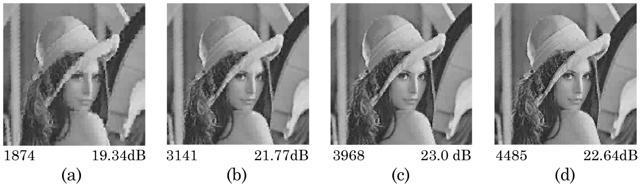
Figure 5. Lena image encoded with (a) 2, (b) 4, (c) 6, (d) 8 NZs at maximum per 16x16 blocks. (Value at bottom left is NZs and SNR is in bottom right)
