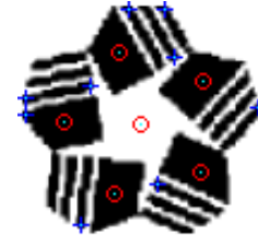
Fig. 7. 15 strongest keypoints of a pattern detected by the Harris corner detector (blue crosses) and the extrema in scale-space of Dog (red circles)
