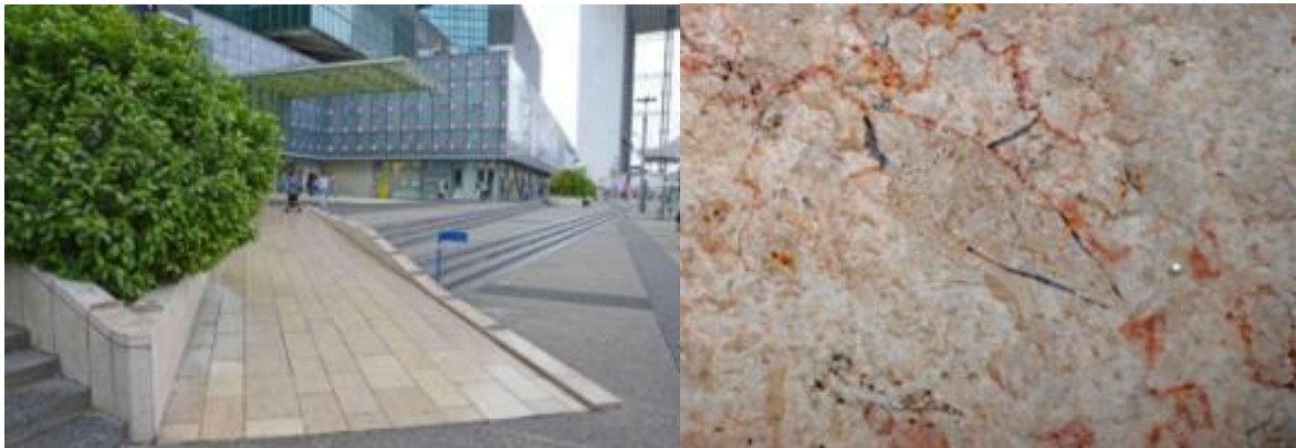
Figure 18 – (left) One of the ramps leading to the Quatre Temps shopping centre, built from Comblanchien limestone from Burgundy. (Right) Comblanchien limestone often has pink veins. These are iron oxides that recrystallized after deposit. Fossils, including the 5 cm long mollusc shell are also present.
