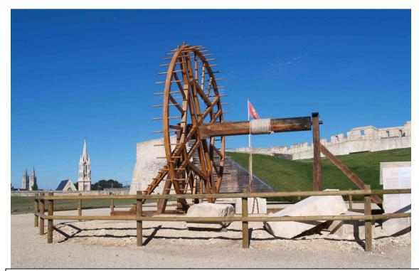
Fig. 14- Winch used to bring to the surface heavy blocks of Pierre de Caen from underground quarries - note the white colour of the stone © <u>D. Peeters</u>
