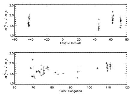
Figure 2. A plot of the ratio of the background obtained using PIA (averaged over all pointings/pixels in a raster)  $\langle F_{\nu}^{PIA} \rangle$  and that from our estimate from a model of the zodiacal background and maps of galactic emission  $\langle F_{\nu} \rangle$  as a function of ecliptic latitude  $\beta$  (top panel) and solar elongation (bottom panel).
