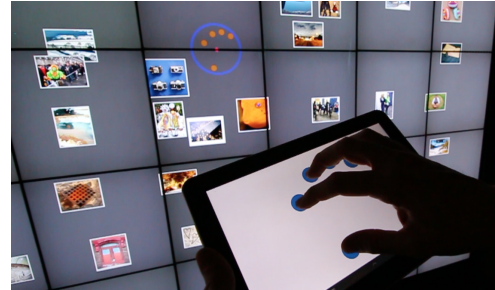
Figure 6. Remote Touch. Projecting touch events from the tablet to the wall with a blue circular area as proxy. The red dot in the center shows the selection point, which corresponds to the center of the tablet.
