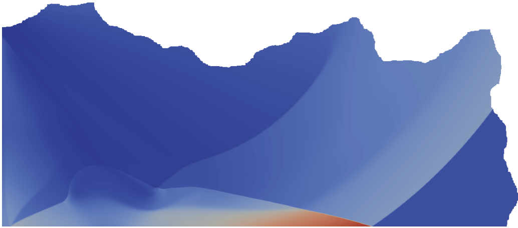
FIGURE 25. Euler equations, shock-square interaction – Density at t = 0.5 – Results obtained with 53 \cdot 10^6 cells, in the area where shock-to-shock interaction occurs, behind the obstacle.
