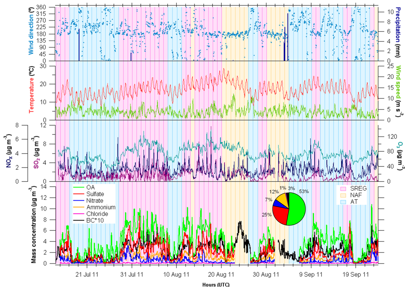
Figure 5. Time series of wind direction, precipitation, temperature, wind speed, concentrations of nitrogen oxides ( \text{NO}_x ), sulfur dioxide ( \text{SO}_2 ), ozone ( \text{O}_3 ), and \text{PM}_{10} chemical species (OA, sulfate, nitrate, ammonium, chloride and black carbon (BC)) in summer (14 July 2011–24 September 2011). Background colors correspond to daily classification of atmospheric episodes (summer regional (SREG), North African (NAF), and Atlantic (AT)) and the pie chart corresponds to the average chemical composition for the summer period.
