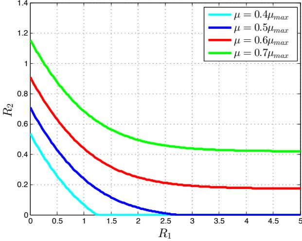
Figure 3: Achievable rates  $R_1$  and  $R_2$  for the Gaussian case with  $X_1 \rightarrow X_2 \rightarrow Y$  for several values of relevance  $\mu$ . The correlation coefficients are  $\rho_{x_1x_2} = \rho_{x_2y} = 0.8$ .
