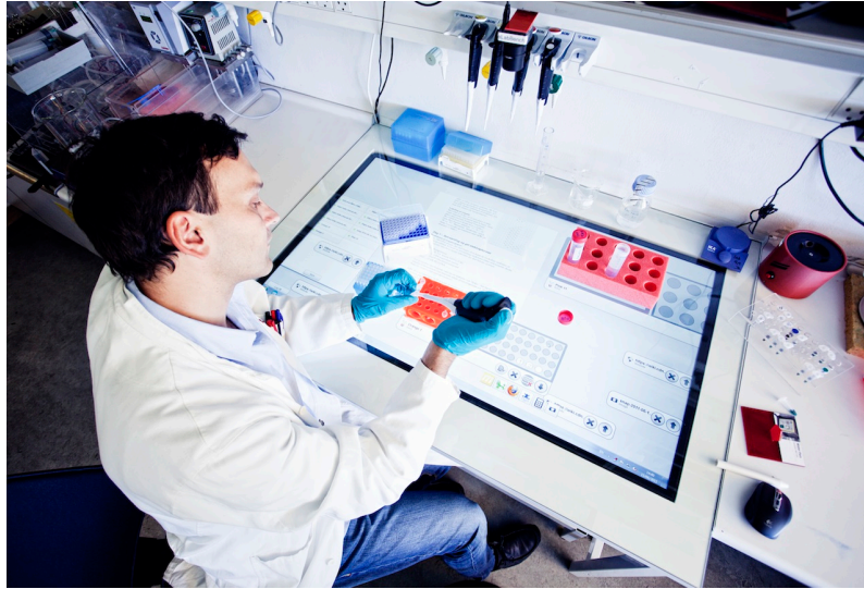
Fig. 7 The eLabBench in use by a biologist conducting a lab experiment organized as an activity. Both physical resources, such as the test tube racks, as well as digital resources, such as research articles and a web-based lab notebook, are included in the activity.
