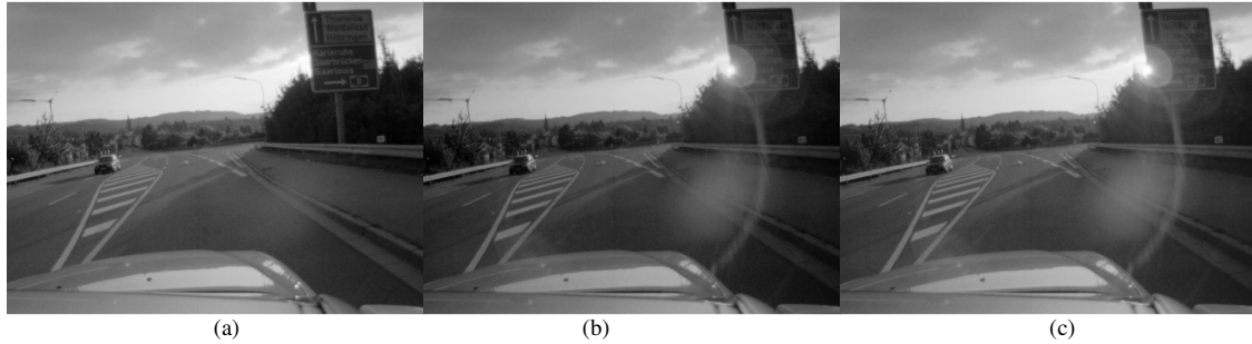
Fig. 3 Tone mapped frames from Sun sequence: a) Frame 222 (Average Intensity: 104.43), b) Frame 223 before flickering correction (Average Intensity: 90.64), c) Frame 223 after flickering correction (Average Intensity: 103.64, k_w=0.01 ).
