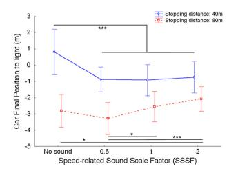
**Fig. 7.** Car final position to light (CPF) as a function of synthesized SSSF for both stopping distances. Error bars represent the 95% confidence interval. Stars represent the level of significance for statistical differences (<sup>\*</sup>p < .05; <sup>\*\*\*</sup>p < .001).
