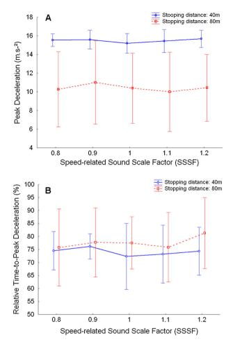
Fig. 6. Peak deceleration (PD; Panel A) and relative time-to-peak deceleration (rTPD in % of the braking duration; Panel B) as a function of realistic SSSF for both stopping distances. Error bars represent the 95% confidence interval.
