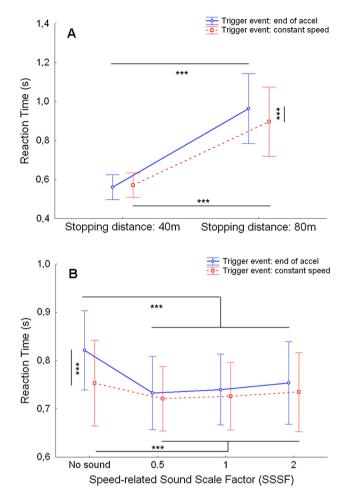
**Fig. 8.** Reaction time to braking (RT) as a function of stopping distance (Panel A) and synthesized SSSF (Panel B) for both trigger events. Error bars represent the 95% confidence interval. Stars represent the level of significance for statistical differences (\*\*\*p < .001).
