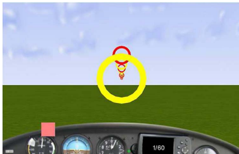
Fig. 1. Screenshot of a typical flying scene created by our home-grown software ICE. The ratio of hit rings over the total number of rings in the trajectory appeared on the cockpit dashboard (e.g., 1/60), and a green or red light indicated whether the last ring had been hit or missed.
