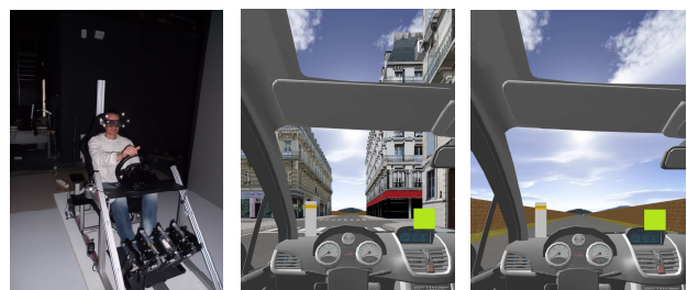
Figure 1: Left: The driving simulator in operation. Center: screenshot of the first part of the simulated environment (urban street). Right: Screenshot of the second part of the simulated environment (field road).
