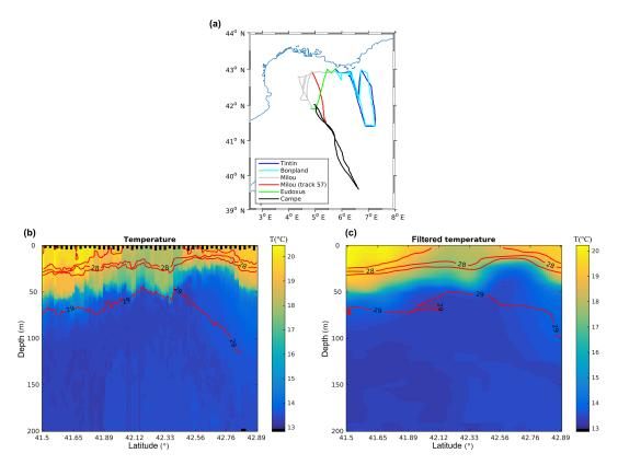
**Figure 5. (a)** Location of the different gliders used in this analysis. In red, the glider Milou section (155 km long) along the SARAL altimeter track 57 from 27 October to 3 November 2014. **(b)** Vertical temperature section from the Milou glider over the upper 200 m. **(c)** Filtered temperature section with cutoff at 30 km wavelength.
