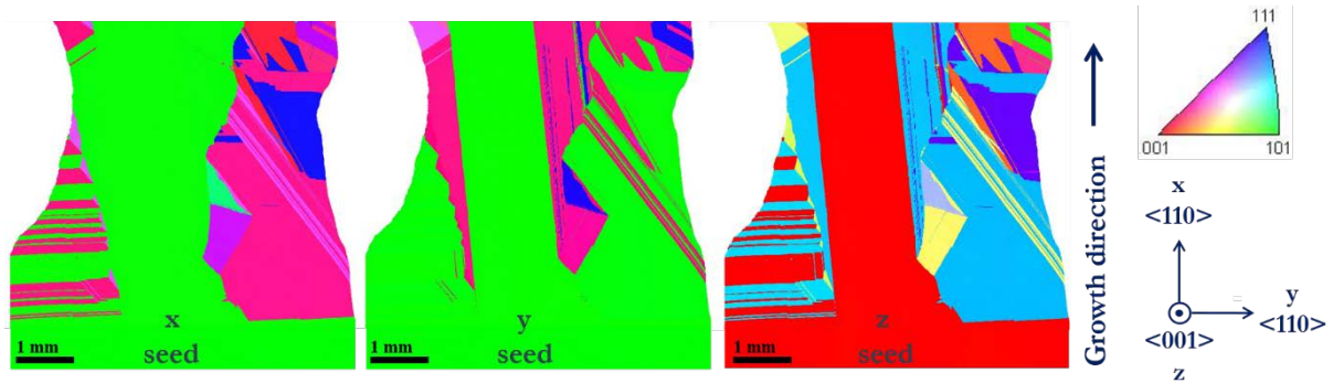
Fig. 2: Crystallographic orientation maps (IPF) of the solidified sample in the x (growth direction), y and z-directions obtained by EBSD ex situ measurements (7 \mu\text{m} step size) after the 13 th melting-solidification cycle performed with an applied temperature gradient G = 30 K/cm and a cooling R = -0.2 K/min.
