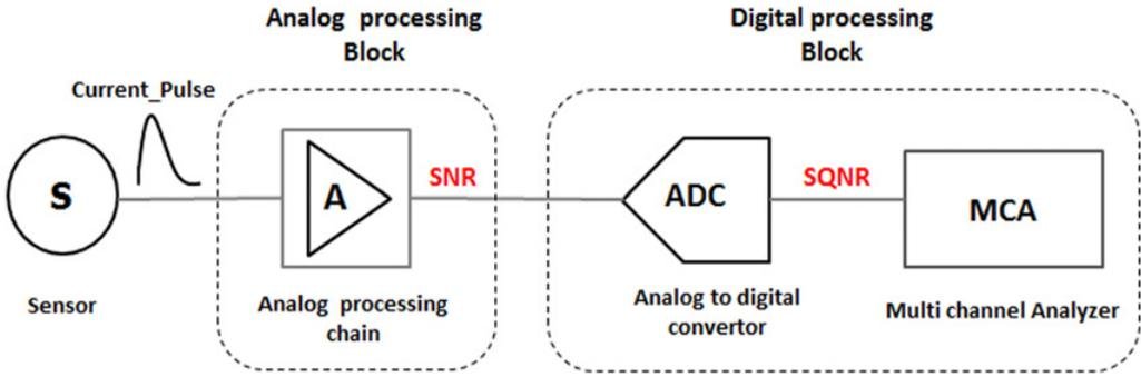
Figure 2. Block diagram of the processing chain.
