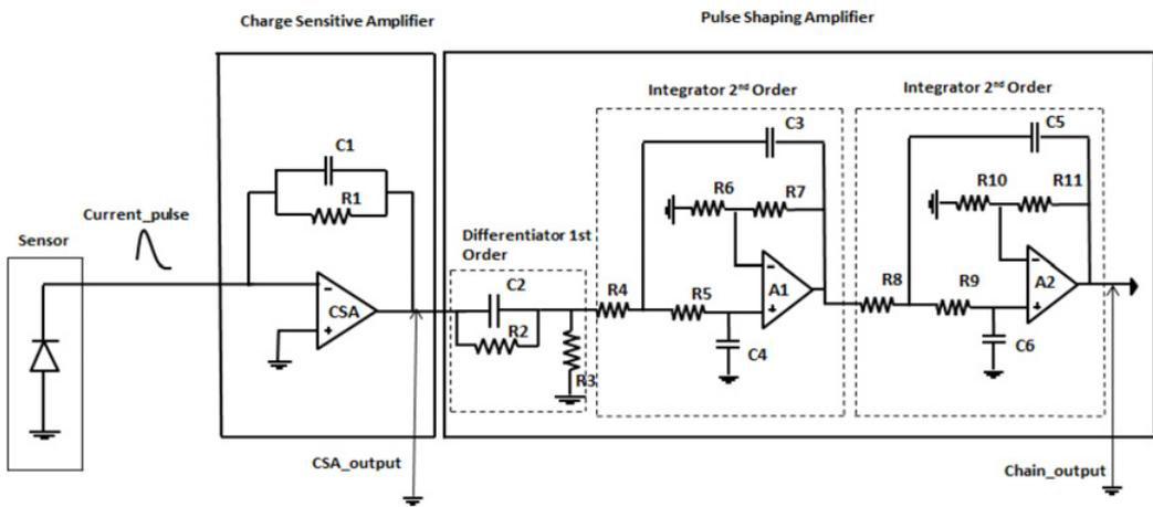
Figure 3. Electrical circuit diagram of the analog signal conditioning (1 channel).
