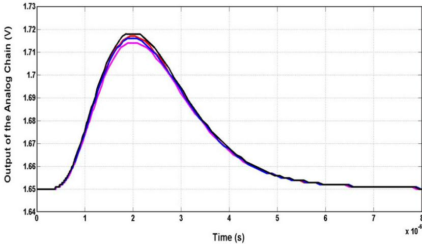
**Figure 7.** Outputs of the analog processing chain corresponding to the input currents shown in Fig. 6 (the currents have the same charge value (65fC)). Same lines colors are considered for each input current and its corresponding output voltage shape.
