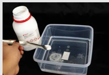
3. Add the selected salt until saturation, i.e. until the salt does not seem to dissolve anymore.
