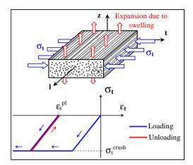
Fig. 3. Crushing principle in the transverse direction.
