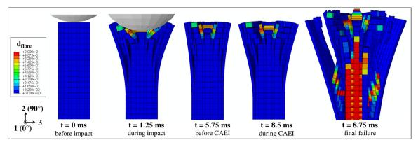
Fig. 12. Section in the (2, 3) plane just under impactor of stacking A impacted at 10 J.
