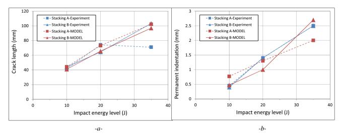
Fig. 7. Experiment/model comparison of maximum crack length (a) and permanent indentation (b) versus impact energy.
