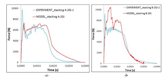
Fig. 6. Experiment/model comparison of the edge impact force/time curves of the stacking A (a) and B (b) impacted 20 J (b).
