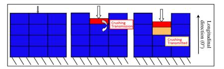
Fig. 4. Crushing transmission principle.
