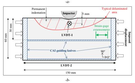
Fig. 1. Experimental set-up of edge impact (a) and guide-rail type connection realised with guiding knives for CAEI (b).
