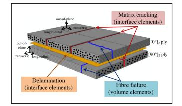
Fig. 2. Modelling of composite damages with the different element types in each oriented ply [15].
