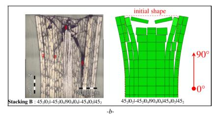
Fig. 5. Experiment/model comparison of cut sections of stacking A (a) and B (b) impacted at 10 J just under the impactor.
