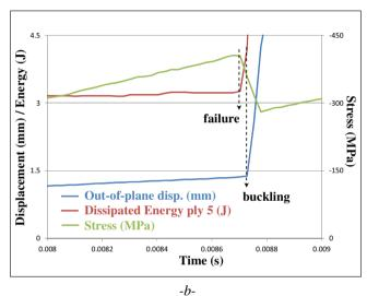
**Fig. 14.** Evolution of out-of-plane, dissipated energy in the 5th ply at 0° and global stress during the 3 phases of the calculation for (a) stacking A impacted at 10 J and (b) zoom on final failure.
