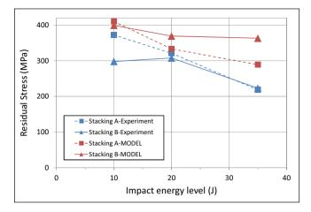
Fig. 15. Experiment/model comparison of the residual stress versus the impact energy level.
