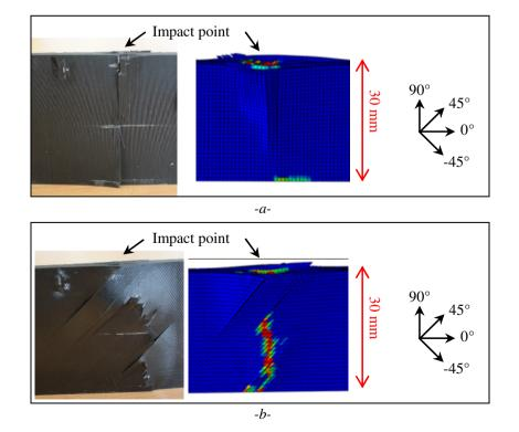
Fig. 9. Experiment/model comparison of the CAEI failure, stacking A (a) and stacking B (b).
