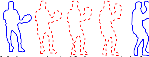
Fig. 10. The backward curve \beta_b^i(t) (left, frame number 1 of Stefan sequence), the forward curve \beta_f^i(t) (right, frame number 5) and the three estimated curves \beta_e^i(t) for \tau = \frac{1}{4}, \frac{2}{4} and \frac{3}{4} (center curves).
