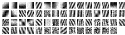
Fig. 2 Dictionary of 59 atoms learnt from Barbara using IBP-DL with a noise level of \sigma_\epsilon = 40 .
