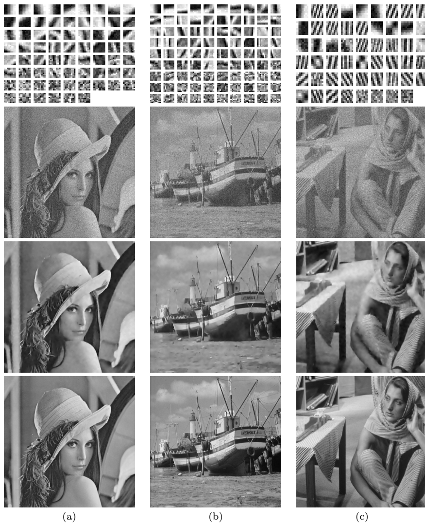
Fig. 9 Illustration of typical denoising results obtained by using IBP-DL on images. From top to bottom are the IBP-DL dictionary, the noisy, the denoised and the original images; (a) Lena, from a PSNR of 20.17 dB to 31.12 dB, (b) Boat from a PSNR of 20.17 dB to 28.92 dB, (c) Barbara from a PSNR of 16.08 dB to 26.34 dB.
