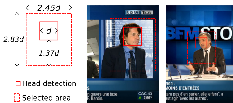
Figure 3. Left: predefined spatial template for the background face selection area given a head detection. Center and right: two examples with head detections and the selected background areas.
