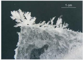
7 Example of crystal growth of ammonium sulphate,  $(NH_4)_2 \cdot SO_{4^{\prime}}$ appearing on a glass plate after three weeks in an 80% RH saline chamber with no cleaning.
