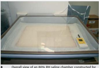
Overall view of an 80% RH saline chamber constructed for flattening documents.
