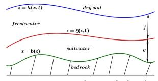
FIGURE 1. Description of an unconfined aquifer
