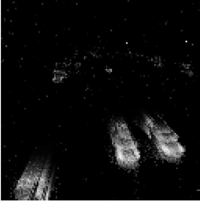
Fig. 5. Input data for the freeway experiment coming from a spike-based camera. The spikes represent a variation of intensity for a given pixel and are generated asynchronously.
