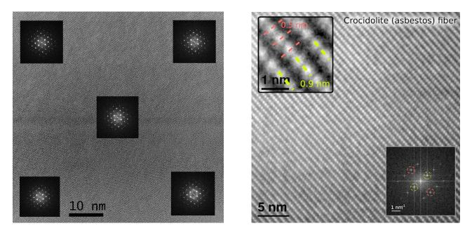
**Figure 2.** Spatial resolutions achieved with the B-corr: (a) **HREM mode:** Dumbles observed in InAs over large field of view with the B-COR associated to the 11mm gap I2TEM objective lens. (b) **Lorentz mode:** 0.5 nm resolution observed in Crocidolite sample
