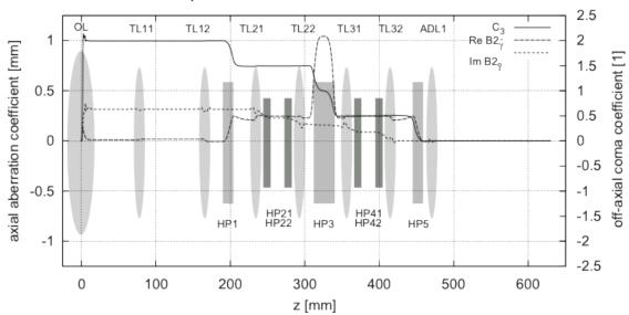
Compensate radial and azimuthal off-axial Coma
