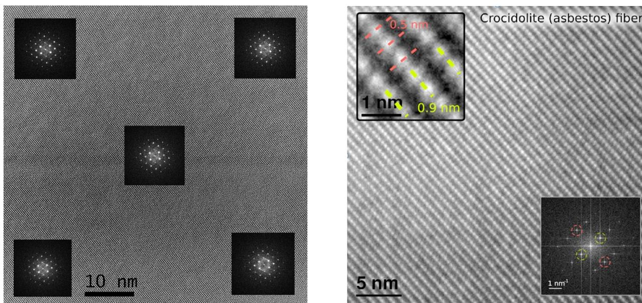
**Figure 2.** Spatial resolutions achieved with the B-corr: **(a) HREM mode:** Dumbles observed in InAs over large field of view with the B-COR associated to the 11mm gap I2TEM objective lens. **(b) Lorentz mode:** 0.5 nm resolution observed in Crocidolite sample
