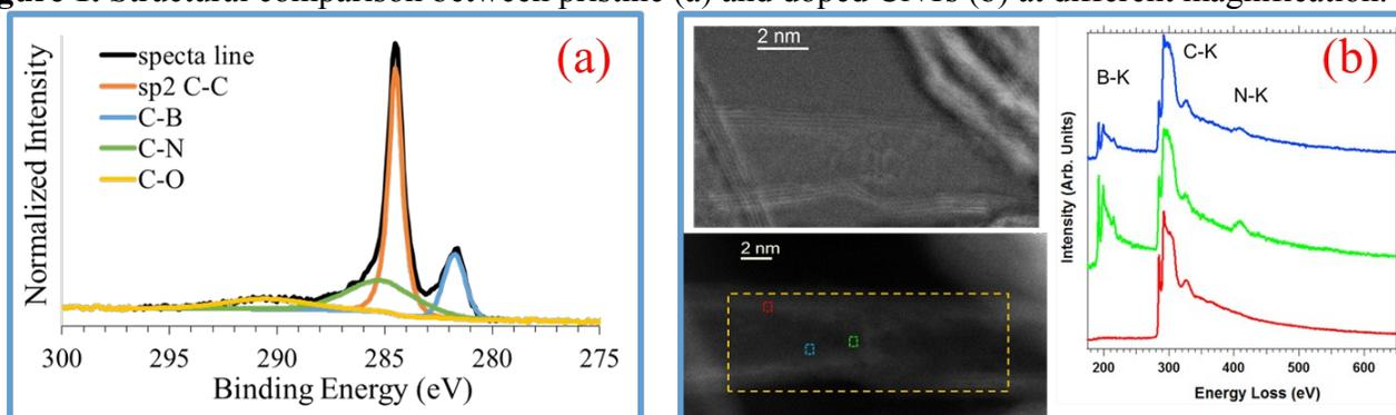
**Figure 2.** (a) XPS spectra of carbon C1s binding energy. (b) Selection of EEL spectra extracted from the spectra image; blue, red and green spectra correspond to the pixels outlined in blue, red and green in bottom left image.
