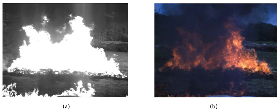
Figure 3. Images of a fire producing dense black smoke in the visible spectrum (a) and in the near infrared spectrum (b).
