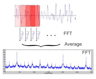
Figure 5. Principle of the FFT computation using Welch's method
