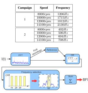
Figure 7. Principle of the proposed method
