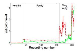
Figure 9. Statistic based (plain) and vibratory (dotted) indicators at 8000*rpm* in campaign 2
