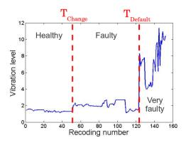
Figure 8. Example of the instant  $T_{Change}$  when the bearing is changed by a faulty one and the instant  $T_{Default}$  when the vibration indicator starts reacting
