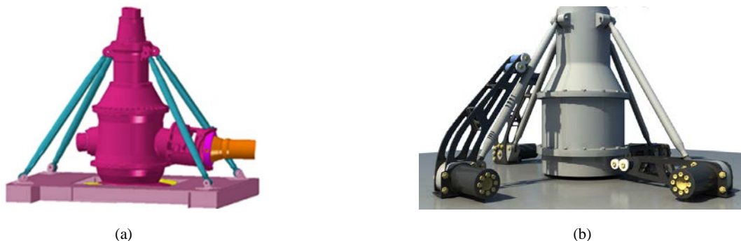
Fig. 2 – (a) Flexible classical MGB-Fuselage suspension, (b) MGB-Fuselage suspension with SARIB system.
