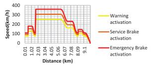
Fig. 16. ERTMS/ETCS supervision limits and braking curves.
