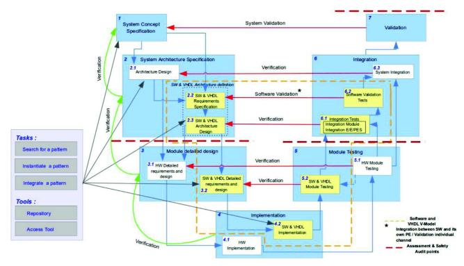
Fig. 20. An overview of the railway reference process model.
