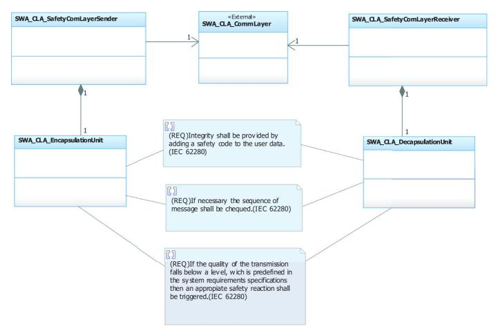
Fig. 8. Black channel for software architecture.
