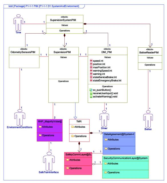
Fig. 22. Overview of the Safe4Rail safety concept.
