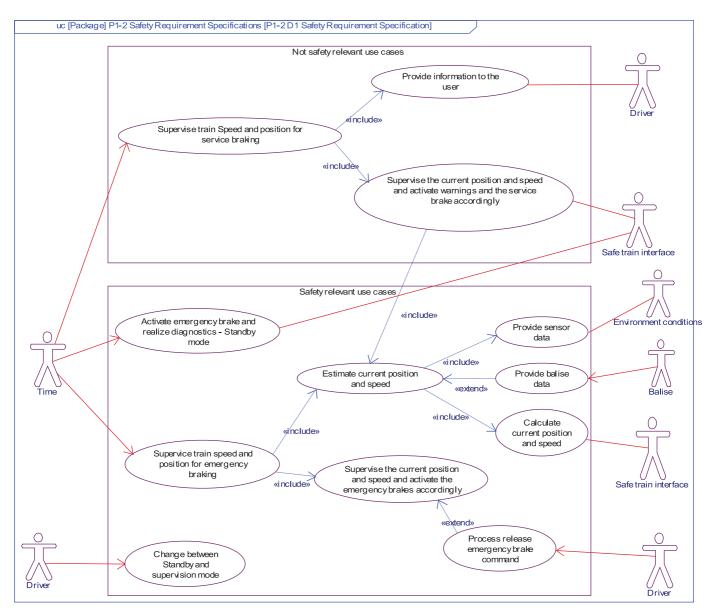
Fig. 18. Part of a Safe4Rail use-case diagram.
