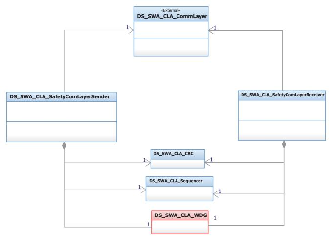
Fig. 9. Railway black channel software architecture.
