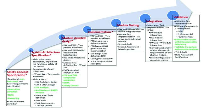
Fig. 2. Reference safety engineering process for railway signaling.
