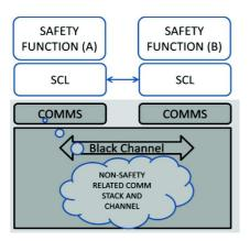
Fig. 7. Safety communication pattern structure.
