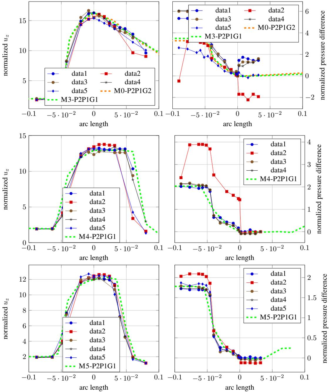
Figure 2: Comparison between experimental data and numerical results for the normalized axial velocity along  $z$  (left) and the normalized pressure difference along  $z$  (right), for  $\mathcal{Re}_t = 500$  (top)  $\mathcal{Re}_t = 2000$  (middle) and  $\mathcal{Re}_t = 3500$  (bottom).
