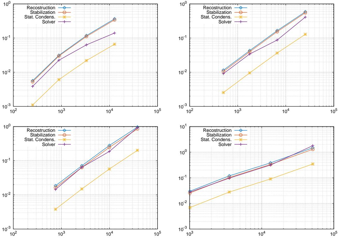
Figure 9: Timings on hexagonal meshes with respect to DOFs using generic data structure (from left to right and from top to bottom:  $k = 0$ ,  $k = 1$ ,  $k = 2$ ,  $k = 3$ ); (violet) crosses: Solver, (red) circles: Stabilization, (blue) diamonds: Reconstruction, (yellow) stars: Static condensation.
