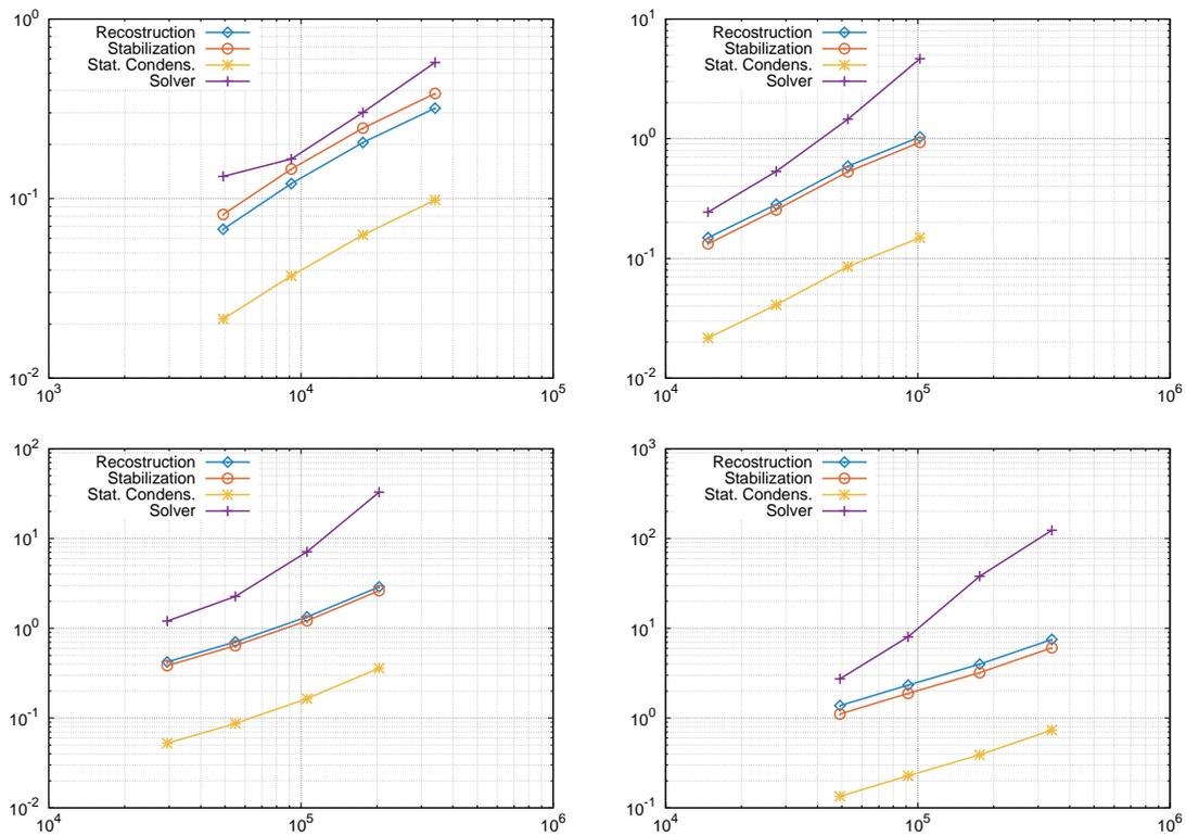
Figure 10: Timings on tetrahedral meshes with respect to DOFs using specialized data structure (from left to right and from top to bottom:  $k = 0$ ,  $k = 1$ ,  $k = 2$ ,  $k = 3$ ); (violet) crosses: Solver, (red) circles: Stabilization, (blue) diamonds: Reconstruction, (yellow) stars: Static condensation.
