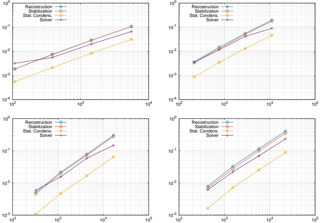
Figure 7: Timings on triangular meshes with respect to DOFs using generic data structure (from left to right and from top to bottom:  $k = 0$ ,  $k = 1$ ,  $k = 2$ ,  $k = 3$ ); (violet) crosses: Solver, (red) circles: Stabilization, (blue) diamonds: Reconstruction, (yellow) stars: Static condensation.
