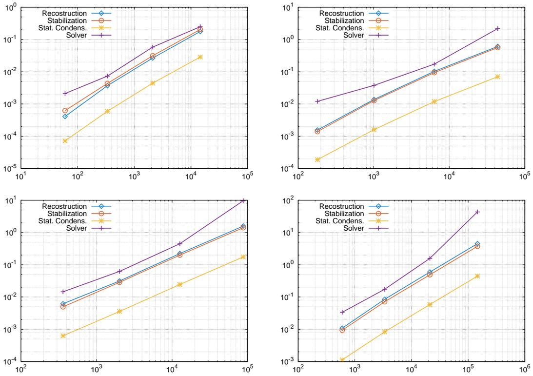
Figure 12: Timings on hexahedral meshes with respect to DOFs using specialized data structure (from left to right and from top to bottom:  $k = 0$ ,  $k = 1$ ,  $k = 2$ ,  $k = 3$ ); (violet) crosses: Solver, (red) circles: Stabilization, (blue) diamonds: Reconstruction, (yellow) stars: Static condensation.
