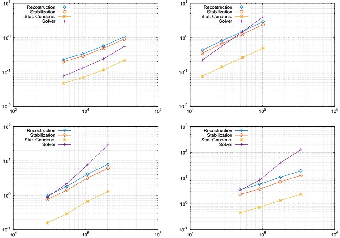
Figure 11: Timings on tetrahedral meshes with respect to DOFs using generic data structure (from left to right and from top to bottom:  $k = 0$ ,  $k = 1$ ,  $k = 2$ ,  $k = 3$ ); (violet) crosses: Solver, (red) circles: Stabilization, (blue) diamonds: Reconstruction, (yellow) stars: Static condensation.
