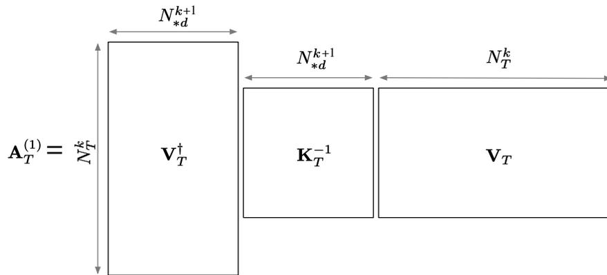
Figure 2: Graphical representation of the computation of the matrix  $\mathbf{A}_T^{(1)}$ . The product  $\mathbf{K}_T^{-1}\mathbf{V}_T$  is carried out with a Cholesky factorization and a subsequent multi-rhs solve.
