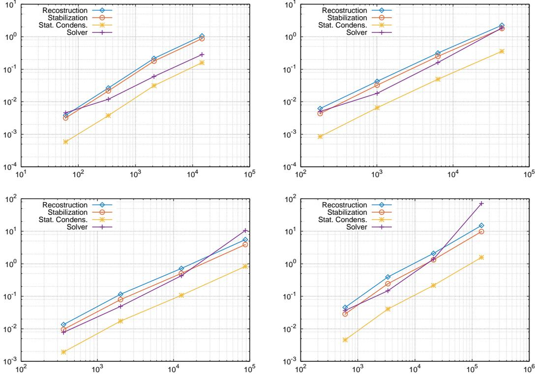
Figure 13: Timings on hexahedral meshes with respect to DOFs using generic data structure (from left to right and from top to bottom:  $k = 0$ ,  $k = 1$ ,  $k = 2$ ,  $k = 3$ ); (violet) crosses: Solver, (red) circles: Stabilization, (blue) diamonds: Reconstruction, (yellow) stars: Static condensation.
