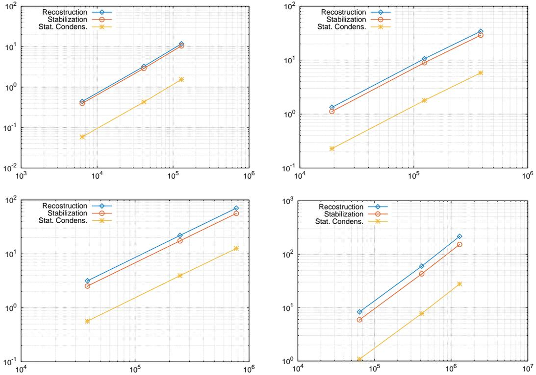
Figure 14: Timings on polyhedral meshes with respect to DOFs using generic data structure (from left to right and from top to bottom:  $k = 0$ ,  $k = 1$ ,  $k = 2$ ,  $k = 3$ ); (red) circles: Stabilization, (blue) diamonds: Reconstruction, (yellow) stars: Static condensation.
