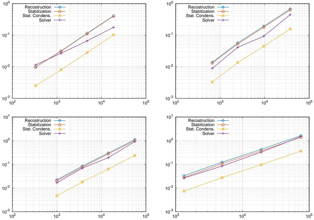
Figure 8: Timings on mixed triangular (50%) and hexagonal (50%) meshes with respect to DOFs using generic data structure (from left to right and from top to bottom:  $k = 0$ ,  $k = 1$ ,  $k = 2$ ,  $k = 3$ ); (violet) crosses: Solver, (red) circles: Stabilization, (blue) diamonds: Reconstruction, (yellow) stars: Static condensation.
