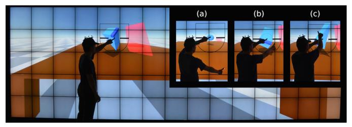
**Figure 1:** 6 degrees of freedom manipulation of a 3D object on a multi-touch wall-sized display combining bimanual interaction and teleportation. The user is performing a xy translation (main picture), z translation (a), roll rotation (b), and pitch & yaw rotation (c).
