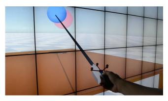
**Figure 3:** For the virtual ray technique, the ray is co-located with the wireless mouse held by the user.
