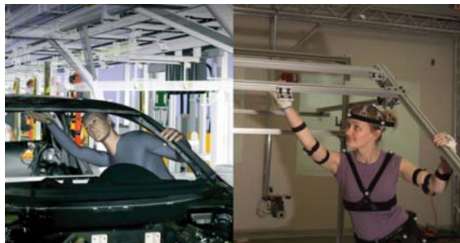
Figure 2: Animation of a DHM using motion capture data, with the Jack software (picture from Jack documentation). The human subject is placed in a physical mock-up of the environment in order to obtain realistic motions.
