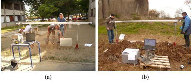
Fig. 3. Ground in situ measurement of surface roughness profile over two sites by laser instrument.
