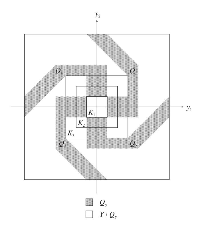
Figure 1: The cross section of the columnar period cell. The regions  $Q_1$ ,  $Q_2$ ,  $Q_3$ ,  $Q_4$  are highly conducting in the plane, and only the central square cylinder  $K_1$  has a non-zero Hall coefficient.
