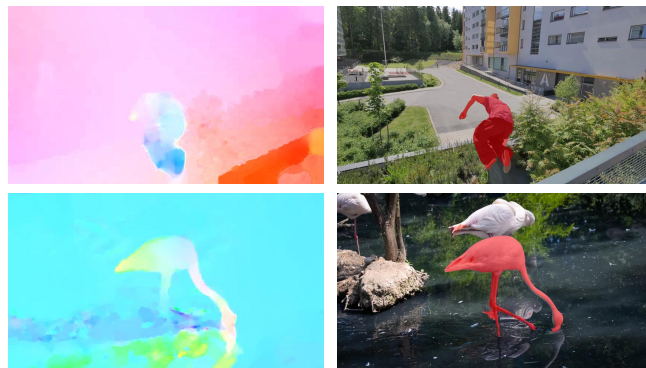
Figure 1. Results on the DAVIS dataset. Left: Optical flow field input to our MP-Net, computed with [6]. Right: Our segmentation result overlaid on the video frame. Note that our approach accurately segments moving objects, and learns to distinguish between object and camera motions (seen in the flow fields).
