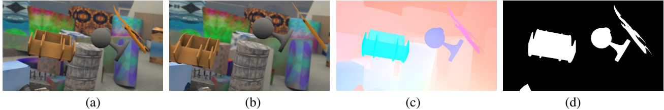
Figure 2. (a,b) Two example frames from a sequence in the FlyingThings3D dataset [26]. The camera is in motion in this scene, along with four independently moving objects. (c) Ground-truth optical flow of (a), which illustrates motion of both foreground objects and background with respect to the next frame (b). (d) Ground-truth segmentation of moving objects in this scene.
