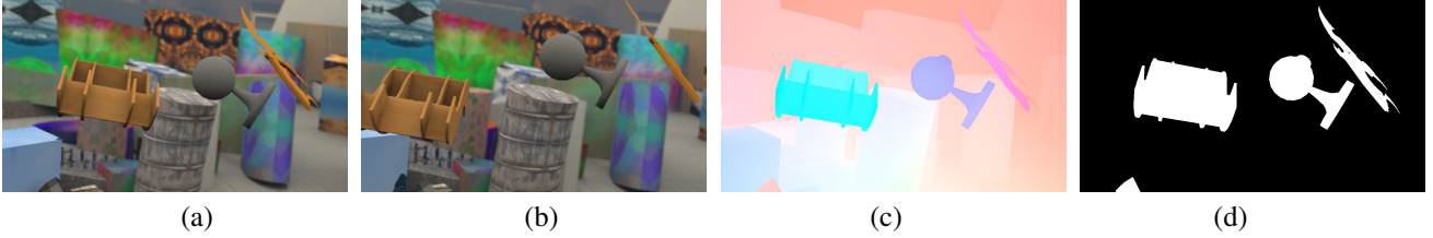
Figure 2. (a,b) Two example frames from a sequence in the FlyingThings3D dataset [23]. The camera is in motion in this scene, along with four independently moving objects. (c) Ground-truth optical flow of (a), which illustrates motion of both foreground objects and background with respect to the next frame (b). (d) Ground-truth segmentation of moving objects in this scene.
