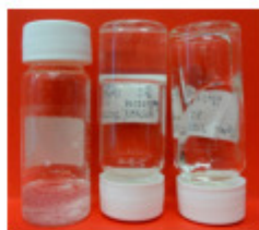
Figure 2. Middle: photograph of the gel formed by a 2/1 mixture (in sticker mole fraction) of 1/2 PDMS at 25 g/L in silicone oil (D5). At the same concentration, 1 is insoluble (left), and 2 PDMS forms a viscous solution (right).
