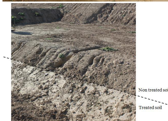
Figure 5. ABOVE : Non treated soil (Zone I) at left hand side, with erosion channels ; lime treated soil (Zone II) at right hand side, with no erosion channel.
