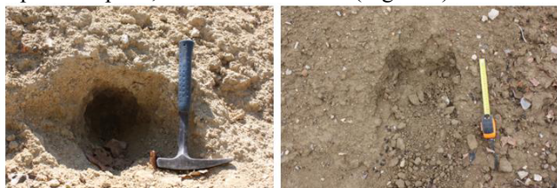
Figure 6. Burrowing animals holes in non treated soil (left) and unsuccessful attempts in lime treated soil (right)
