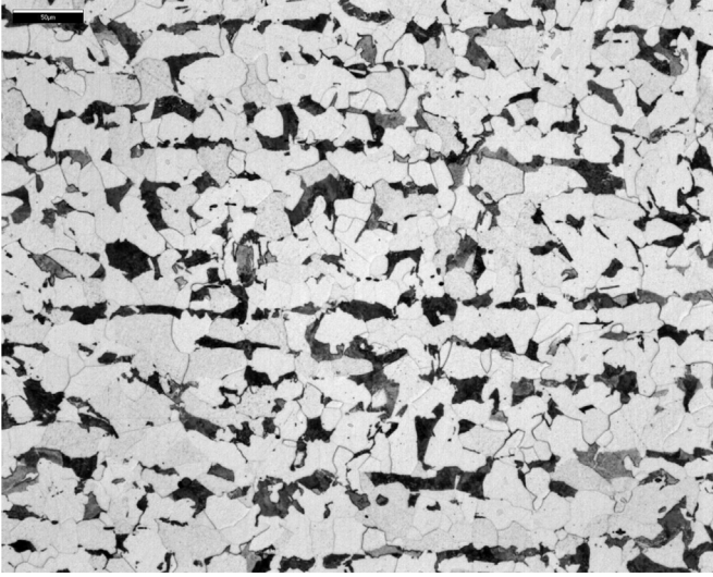
Fig. 1. Microstructure of A48 steel.
