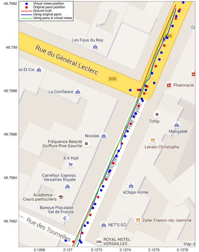
Fig. 1. The output from a single localization run using original Street Views and synthesizing virtual views: The trajectories obtained with/without virtual views are plotted in green/blue respectively. The ground truth in red line is recorded by a centimeter-level real-time kinematic GPS (RTK-GPS).
