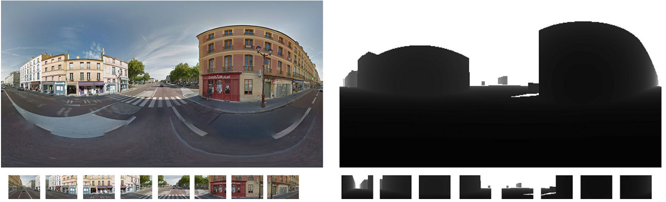
Fig. 3. An example of Street View panorama (top-left) and its associated depth map (top-right) at location [48.799133, 2.127752] in Versailles, France. The below 8 rectilinear images and depth maps are extracted from the above ones by the back projection. The 8 virtual pinhole cameras are configured similarly to the vehicle’s camera, including the same focal length and image size. It creates overlapping views.
