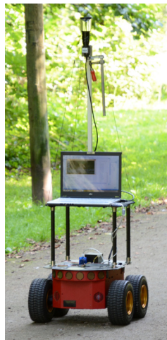
(d) Pioneer 3-AT robot equipped with the hypercatadioptric camera.
