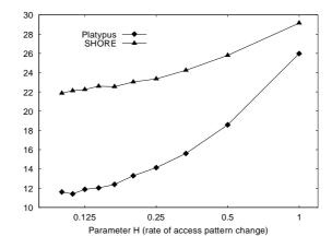
Fig. 5. Traversed objects results. The x-axis is in log<sub>2</sub> scale. The minimum and maximum coefficients of variation are 0.005 and 0.037, respectively.
